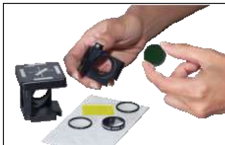
Figure 3 Installing a filter set in the removable holder
