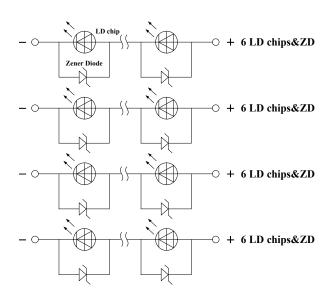
This model does not have a Photo Diode. This model has a Zener Diode built in as a protection circuit against static electricity.
